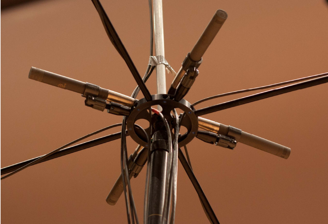
FIGURE 5 – CLOSE-UP OF CENTRAL QUAD SQUARE USING THE ‘WILLIAMS STAR’ MICROPHONE ARRAY SUPPORT SYSTEM. (PHOTO BY MICKAEL KENNESSI)
